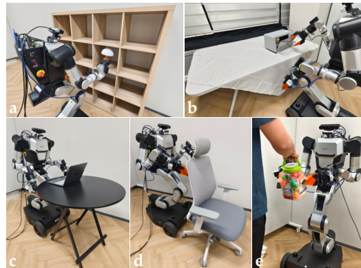
Figure 13: (a) Lamp Retrieval (b) Open Microwave (c) Use Laptop (d) Push Chair (e) Toybox Handover
