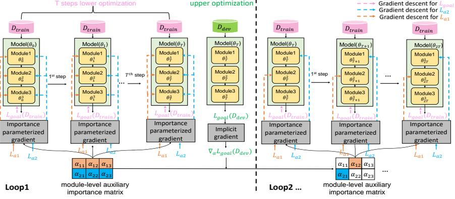
Figure 2: The module-aware optimization method for auxiliary learning. In each loop, the lower optimization is conducted for  $T$  times followed by one-step upper optimization. In the example, in Loop1, the two auxiliary losses  $L_{a1}, L_{a2}$  update all modules equally. After Loop1 optimization,  $L_{a1}$  is only important to module2 and is used for updating module2 while  $L_{a2}$  only for module1.
