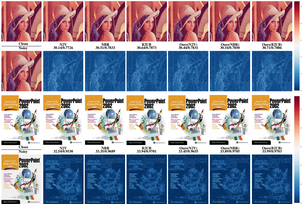
Figure 9: Visual comparison of denoising sRGB images in the setting of Gaussian noise ( \sigma \in [5, 50] ) on SET14. For better viewing, we show the difference between the denoising results and Clean in colour.
