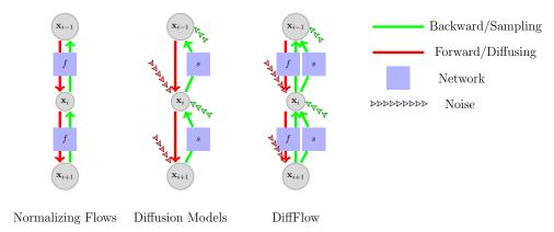
Figure 1: The schematic diagram for normalizing flows, diffusion models, and DiffFlow. In normalizing flow, both the forward and the backward processes are deterministic. They are the inverse of each other and thus collapse into a single process. The diffusion model has a fixed forward process and trainable backward process, both are stochastic. In DiffFlow, both the forward and the backward processes are trainable and stochastic.
