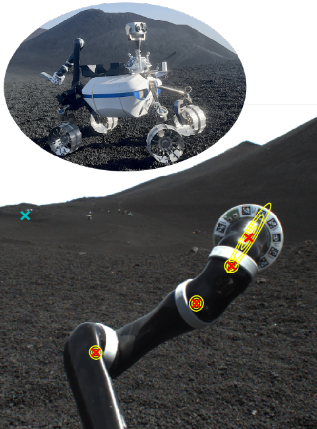
Fig. 1: top – The Lightweight Rover Unit (LRU) on Mt. Etna during the ARCHES field test [1]. bottom – The middle camera on the robot’s head records the movement of the Jaco2 arm. Detected keypoints (red), the corresponding uncertainty ellipses (yellow), and detected false positives (petrol) in the background are shown.
