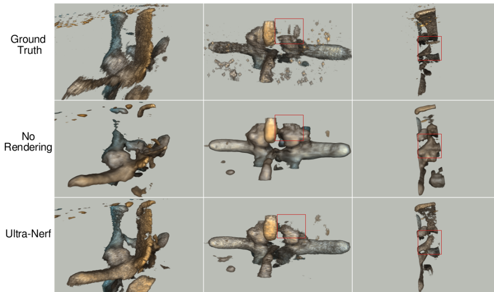
Figure 6: Compounded volumes: without rendering (middle row) the model is not aware of the viewing direction hence occluded parts of the lamina are reconstructed (red). By adding the rendering function, we introduce view-direction dependency needed to reconstruct anisotropic phenomena.
