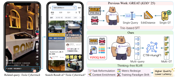
Figure 1: Bottom-bar query suggestion on Kuaishou and key improvements to prior work: V2V2Q RAG for context enrichment, multi-query output with multi-query ground truth, and thinking-free RLVR optimized by proposed metric CTR-HungF1.
