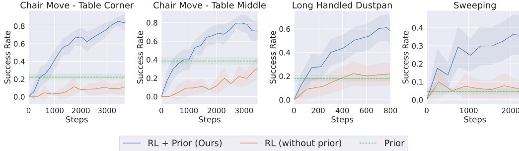
Figure 4: Continual training improvement: Success rate vs number of samples for ours, only RL and only prior. Note that we use our task-relevant autonomy approach with all methods. We see that our approach continuously improves with experience across tasks, learning much faster than RL without priors, and attaining significantly higher performance than just using the prior.
