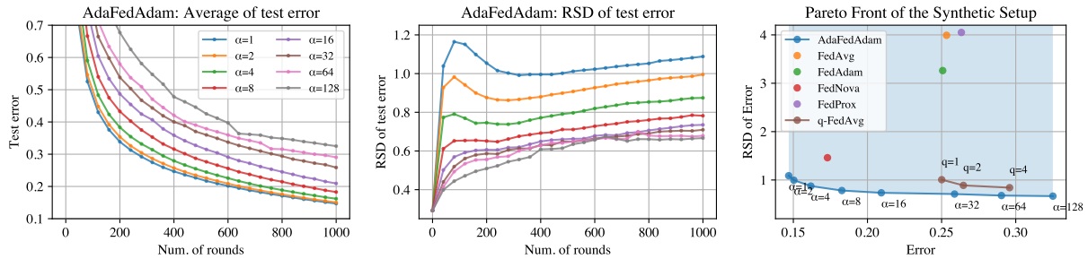
Figure 3: Left : Training curves of AdaFedAdam with different \alpha on the Synthetic setup. Middle : RSD of local error of AdaFedAdam with different \alpha on the Synthetic setup. Right : Pareto Front of the Synthetic setup formed by AdaFedAdam with different \alpha . By adjusting values of \alpha , the trade-off between the convergence and the fairness can be observed together with the suboptimality of other federated algorithms.
