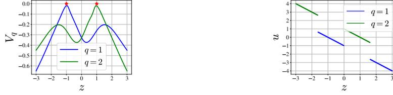
Figure 1: Left, the approximate value function  $\hat{V}_1$ , in blue, and  $\hat{V}_2$ , in green, for the policies  $\pi_1$  and  $\pi_2$ , respectively. Right, the resulting control policy by applying the supervisory policy  $Q^*$ . The setpoints  $\mathcal{Z}^*$  are denoted by the red stars.
