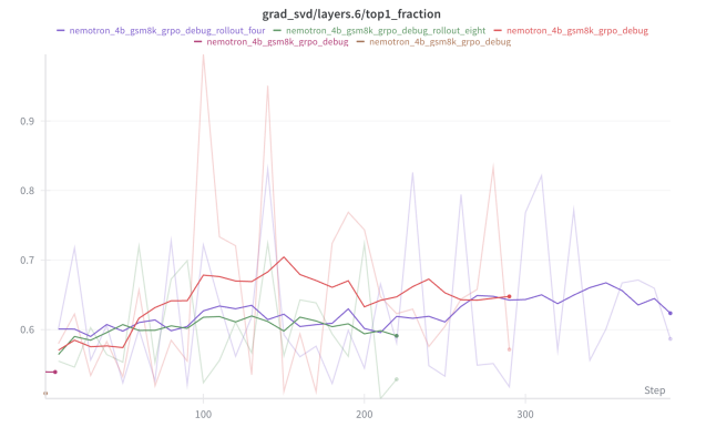
Figure 2. Top-1 singular value fraction ( \sigma_1^2 / \sum_i \sigma_i^2 ) across training. R = 4 shows the highest concentration, while R = 8 diffuses energy across more components. This non-monotonic pattern is explained by the interplay between advantage concentration and trajectory score diversity.
