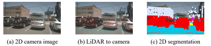
Figure 4: Using the projection of point clouds to image to generate pseudo-labels for 2D image segmentation. (a) The original 2D image. (b) Projection of point clouds to 2D image. (c) Pseudo-labels generated by up-sampling.
