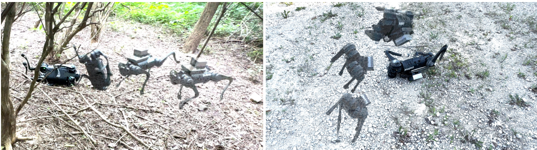
Figure 8: Failure case of the Procedural Generation Curriculum policy due to rapid movements.
