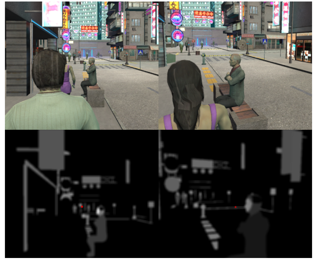
Figure 9: One agent walks behind another and both see the same man sitting on a bench. On the right the man's saliency is lower due to saliency decay during fixation. Top: RGB view from behind the agent so that the head orientation is visible. Bottom: Saliency map from the agent's POV using the particle model.
