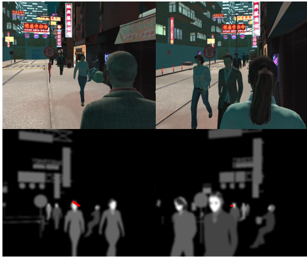
Figure 8: Two agents walking while using the particle gaze model simultaneously. Top: RGB view from behind the agent. Bottom: Saliency map from the agent's POV. The small red line in the center of the saliency map indicates the current direction of the particle gradient.
