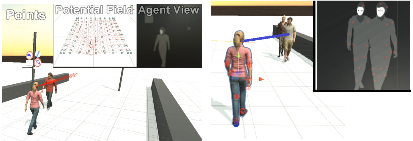
Figure 6: Comparison of target selection between the two models. Left: Particle model, which drives gaze in the direction of the potential field gradient. Right: Probabilistic model target selection. Red circles indicate potential target locations, which once selected will trigger a saccade.
