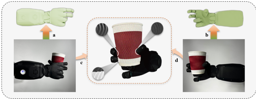
Figure 2: By real-time linking the degrees of freedom of each joint with actual dexterous hand movements and the simulation platform, the RH8D grasping actions are precisely extracted. a, b: From reality to simulation; c, d: Enlarging the clear 2D tactile information at the dexterous hand grasping contact fingertips.
