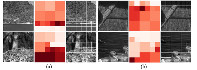
Figure 7: Visualization of two sets of scale-aware sampling (right) and scale-variable adaptive sampling rate allocation (shown as the heatmap in the middle) with the corresponding original image (left).
