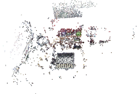
Figure 4: Selected Keypoints with the Highest Matching Rate in chess scene. These key points encompass nearly all regions of the scene that are readily observable while discarding areas with ambiguous interpretations.
