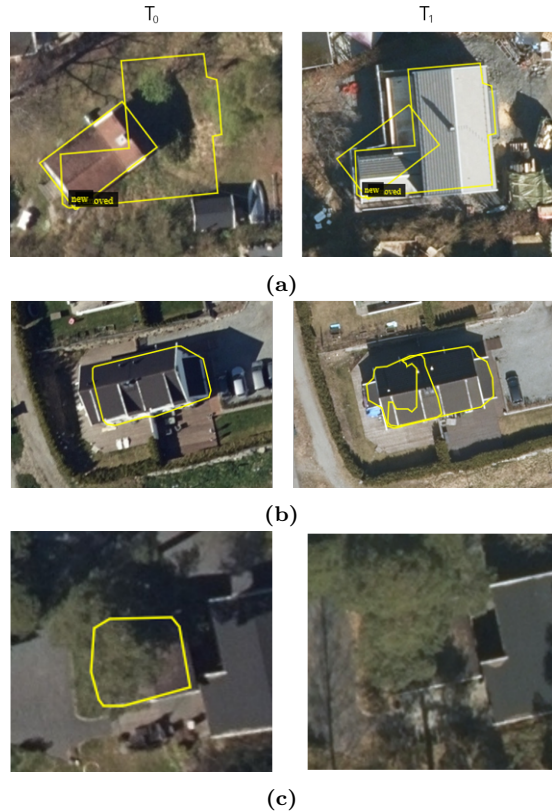
Figure 2. Challenges in post-detection mask comparisons: a) An instance showcasing spatial overlap between a new and a removed building. b) A demonstration of T0 and T1 output mask inconsistency. c) A scenario where discerning the building structure proves challenging due to external factors, here vegetation.
