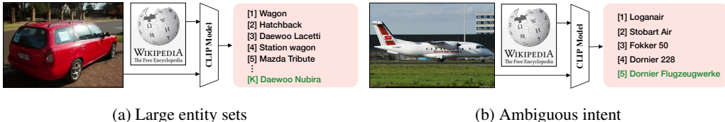
Figure 2: Why is OVEN challenging? We show that CLIP cannot solve OVEN out of the box. We ran CLIP to encode images from standard recognition datasets and retrieve Wikipedia titles from 100K Wikipedia entities. Left: (a) As the # of labels become large, difficult negatives start appearing. For example, DAEWOO LACETTI does not belong to the original label set. Right: (b) Intents can be ambiguous— DORNIER 228 is the model and DORNIER FLUGZEUGWERKE is the manufacturer.
