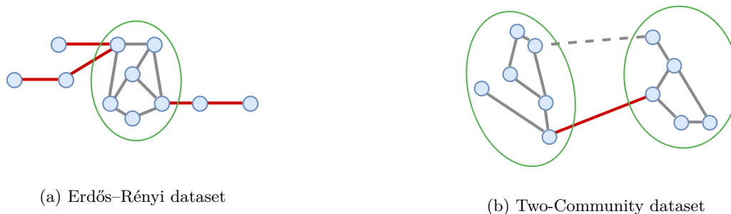
Figure 4: Illustration of two datasets generated for measuring the performance of a model on Bridges task. (a) The dataset generated by the CLRS benchmark. (b) We generate a two-community dataset for a stricter measurement of the Bridges task. The dashed edge is present in one graph and absent in the other graph of the pair. Red edges show the target bridges. Green ovals show connected components. A model with 98% OOD F1 score on the dataset (a) fails to detect the bridge between the two communities of the dataset (b).
