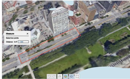
(b) The model distance (3.47 millimeters) between locations *Point 2* and *Point 3*.
