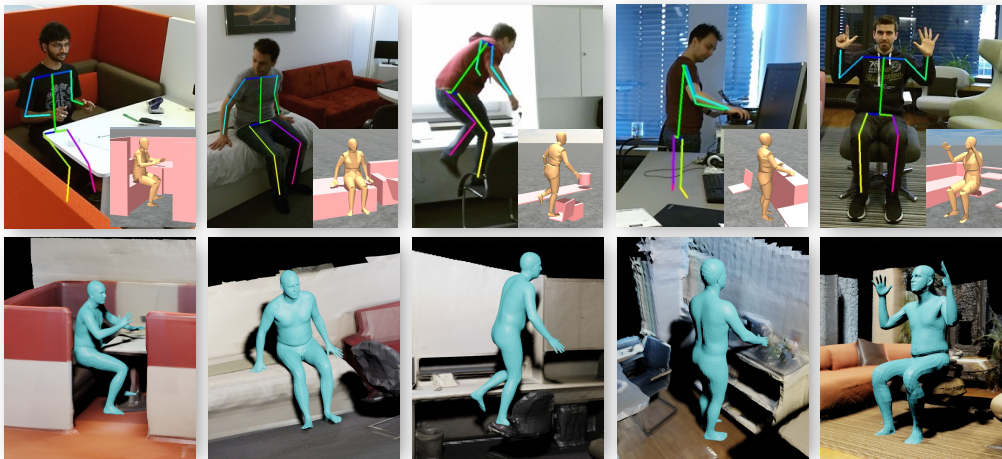
Figure 1: From a monocular video input in a known scene, we estimate 3D absolute body pose by controlling a simulated character to match 2D observation in a sequential manner.
