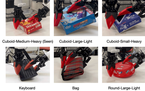
Figure 6: Selected objects of varying sizes and weights requiring occluded grasping are used to evaluate COMBO-Grasp in the real world.
