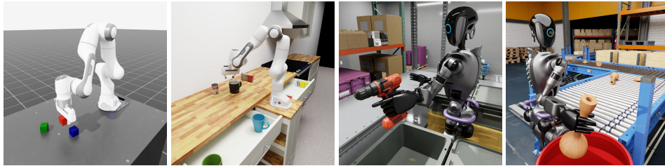
Figure 3: Environments introduced to evaluate policies’ spatial memory. From left to right: Cube Stacking : stack three cubes (initial cube positions are randomized), Mug in Drawer move mug into drawer containing mugs (positions of objects on kitchen counter are randomized and the destination drawer position is permuted), Drill in Box : put hand drill into open box (drill position is randomized and open/closed boxes are permuted), Stick in Bin : put candlestick into bin (stick and bin positions are randomized). In all tasks, policies are provided a single ego-centric camera view from which the entire task space cannot fit into the FOV.
