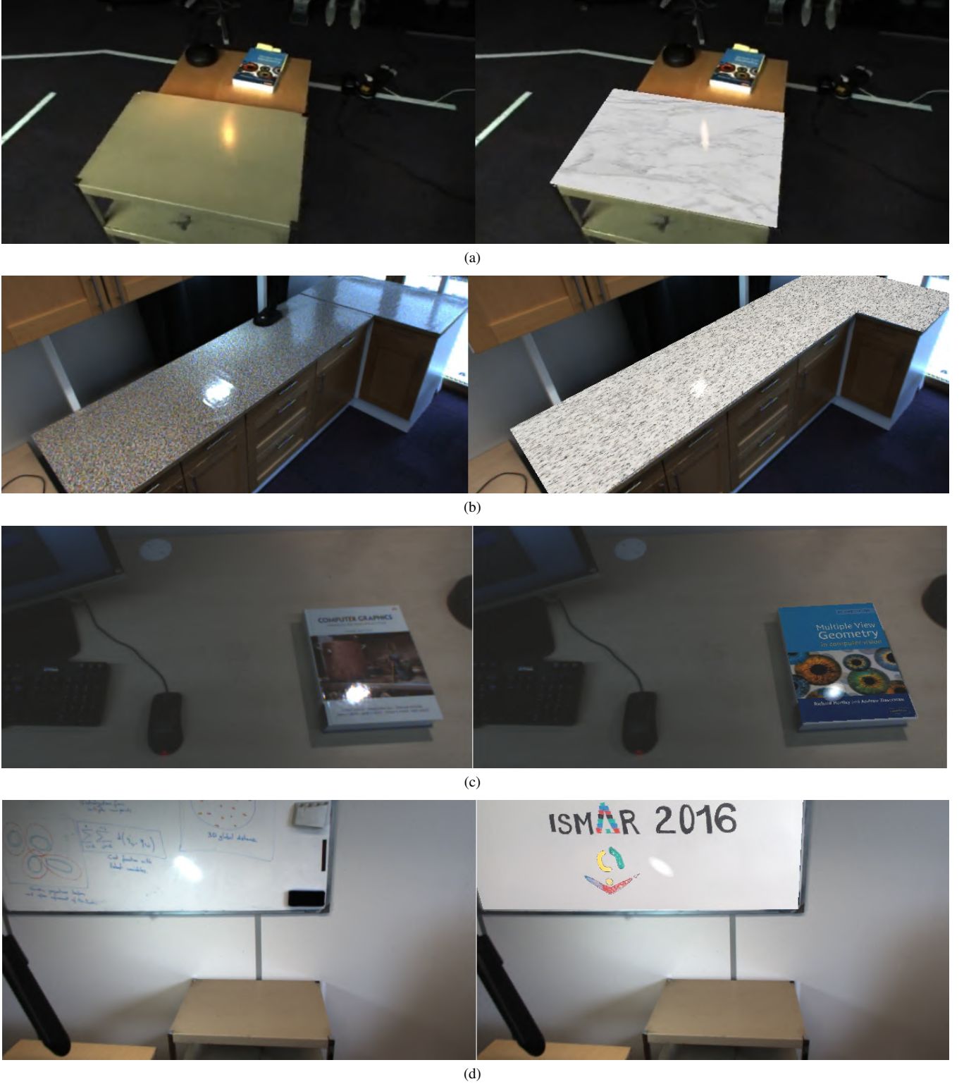
Figure 7: Retexturing method illustrated on the light bulb/steel table sequence (a) by using a marble texture, the fluorescent lamp/kitchen counter sequence (b) using a rock texture, the light bulb/book sequence by switching the book cover (c) and the fluorescent lamp/whiteboard by changing the content on the whiteboard (d). To simulate the specularly, we used a Gaussian function and transformed it onto the plane surface using our specularly prediction to compute the transformation. The color of the specularly is computed from the specularities detected in the images used for the quadric reconstruction. Without considering the diffuse term on the texture, we can realistically change the texture of the planar surface using only the specular term predicted by JOLIMAS. The retexturing sequences can be found in the supplementary materials
