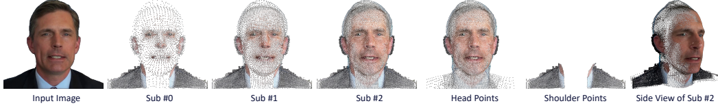
Figure 2: As the subdivision level increases, the resolution of head meshes and features are progressively refined. The Gaussians for the head and shoulders are predicted separately and integrated via cross-region combination. The head Gaussian counts for Sub #0, Sub #1, and Sub #2 are 5K, 20K, and 80K, respectively. See Table 5 in the appendix for more details.
