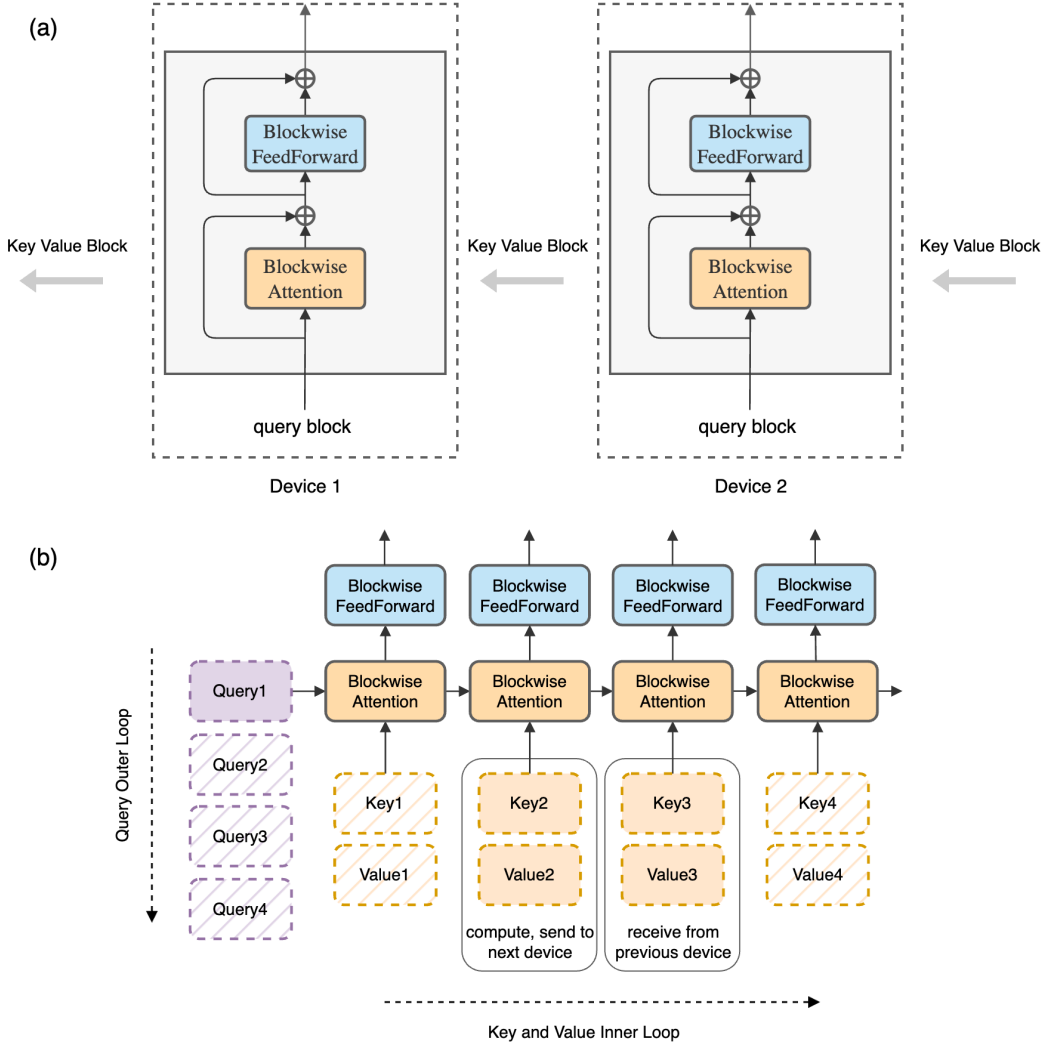
Figure 2: Top (a): We use the same model architecture as the original Transformer but reorganize the compute. In the diagram, we explain this by showing that in a ring of hosts, each host holds one query block, and key-value blocks traverse through a ring of hosts for attention and feedforward computations in a block-by-block fashion. As we compute attention, each host sends key-value blocks to the next host while receives key-value blocks from the preceding host. The communication is overlapped with the computation of blockwise attention and feedforward. Bottom (b): We compute the original Transformer block-by-block. Each host is responsible for one iteration of the query’s outer loop, while the key-value blocks rotate among the hosts. As visualized, a device starts with the first query block on the left; then we iterate over the key-value blocks sequence positioned horizontally. The query block, combined with the key-value blocks, are used to compute self-attention (yellow box), whose output is pass to feedforward network (cyan box).
