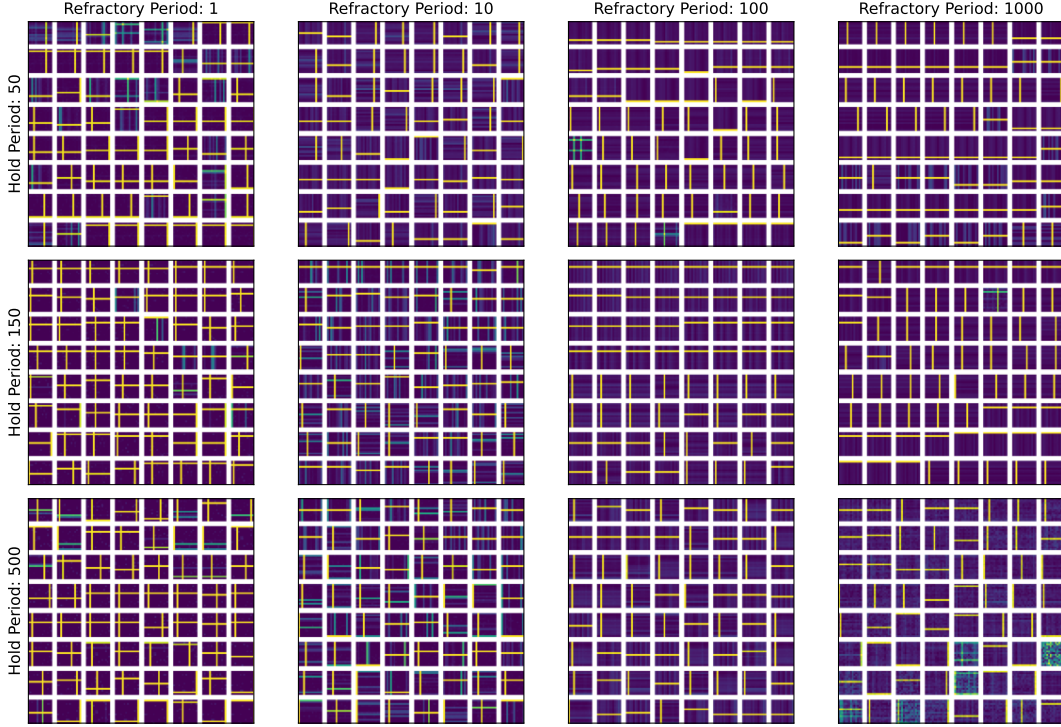
Figure C.5: Receptive fields of top 100 most active neurons for different refractory periods of the asynchronous model. Models were simulated with different presentation (holding) times, quantified by Euler steps (rows)
