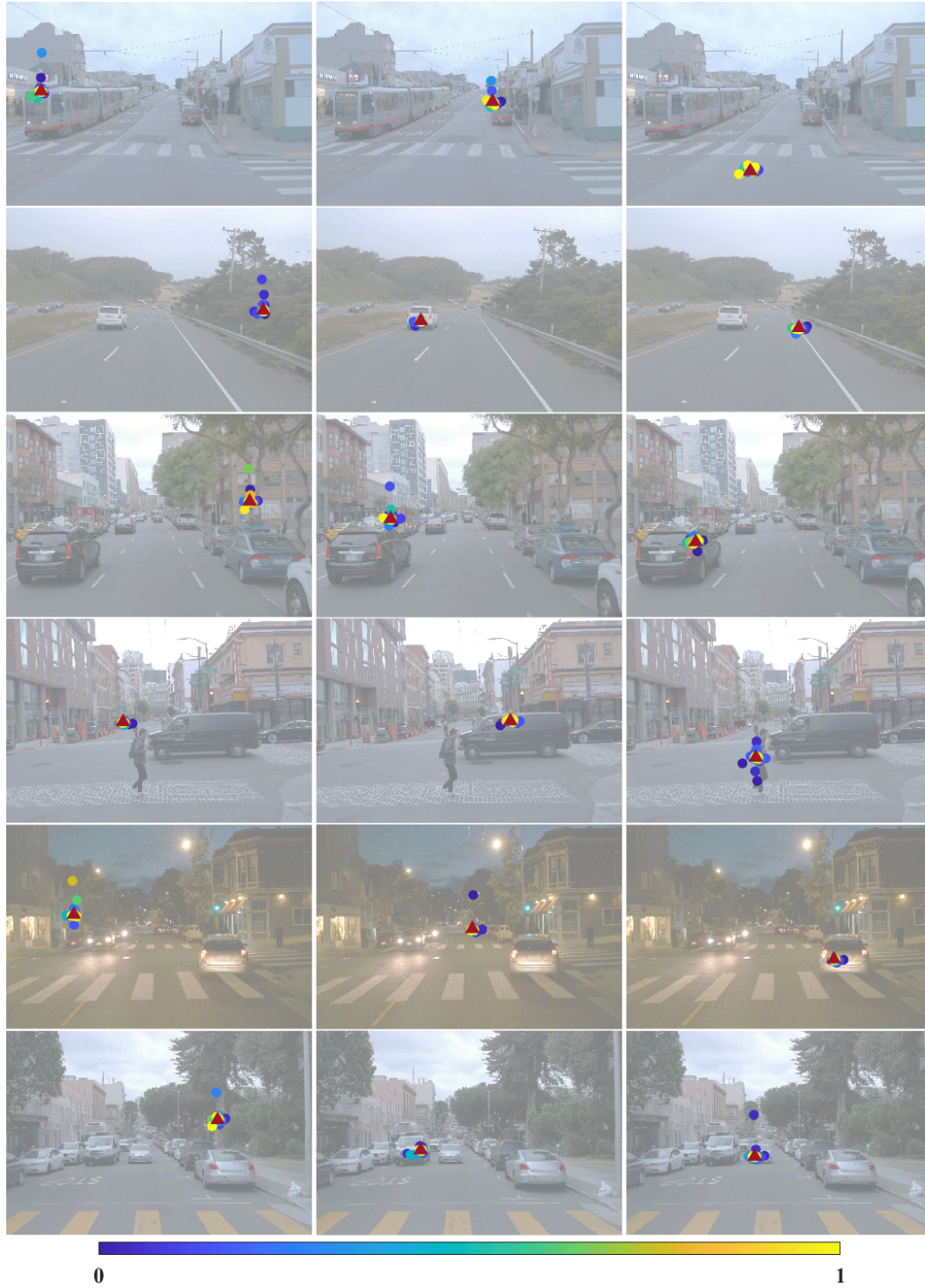
Figure 12: Visualization of the deformable attention model. Red triangle indicates the reference point, i.e., the 2D projection of the query. Dots represent the predicted sampling locations, and they are colored according to their attention scores.
