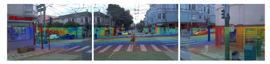
Figure 9: Visualization of the LiDAR point cloud and camera images. Points are colored according to their range value. Best viewed zoomed in.
