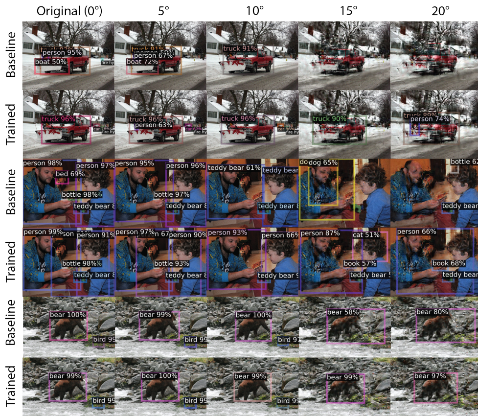
Figure 3: Training improves object detection on Uniform TTM images. Faster-RCNN R50 FPN trained from scratch on peripherally transformed images retains more stable predictions with more accurate bounding boxes as eccentricity increases when compared to the baseline Faster-RCNN R50 FPN model.
