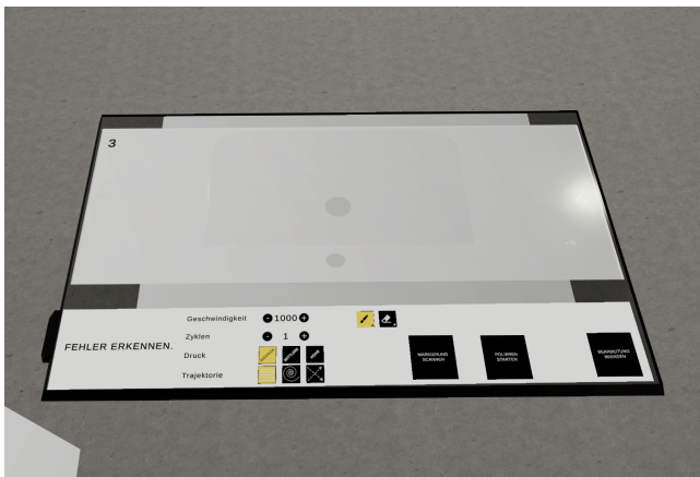
Figure 2: User interface for editing the polishing parameters of the robot, where the polishing speed, the number of polishing cycles, the pressure and the type of trajectory can be adjusted for each area.
