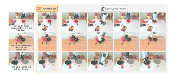
Figure 4: Example real-world HAMSTER rollouts demonstrate its strong performance in novel scenes achieved by leveraging VLMs' generalization capabilities and the robust execution of low-level 3D policies.
