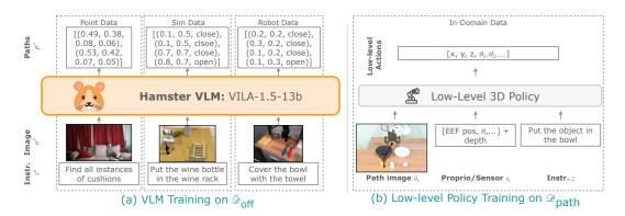
Figure 6: (a): Examples of training data in  $\tilde{\mathcal{D}}_{off}$  used to train HAMSTER's VLM. (b): The data used to train HAMSTER's low-level policies.
