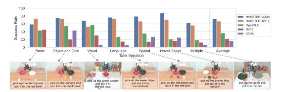
Figure 3: Quantitative evaluation results on a real-world robot, evaluated across different axes of generalization. Across all generalization axes, HAMSTER outperforms monolithic VLAs and 3D imitation learning.
