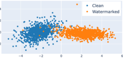
Figure 4: Two-dimensional visualization of the latent space showing the linear separability of watermarked and non-watermarked images. The horizontal axis is obtained by linear discriminant analysis (LDA), while the vertical axis is a random projection.
