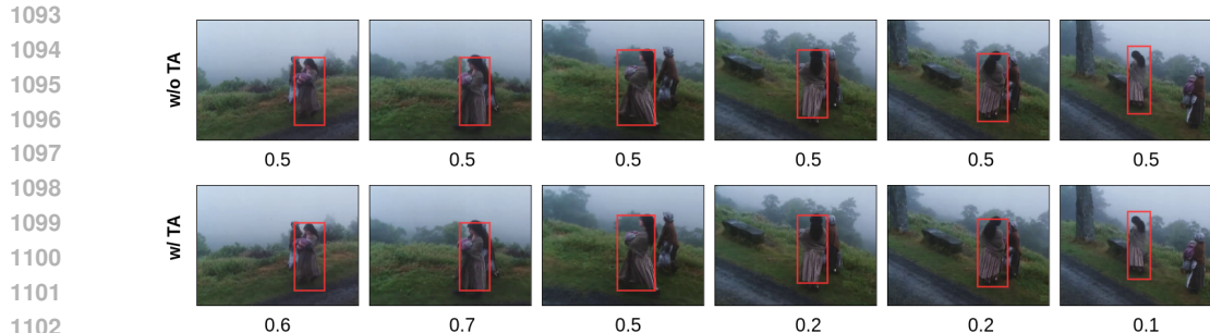
1103 Figure 9: Effect of Temporal Attention: Without temporal attention (w/o TA) in first row, we 1104 observe that each frame gets equal weight, however, utilizing temporal attention (w/ TA, second row) 1105 increases weight on key frames and decrease weight for non-important frames in relation to query. 1106 Query: The woman holding the child walks to the side of a stone 1107 bench stops hands the child to the woman next to her and walks to 1108 the front of the stone bench
