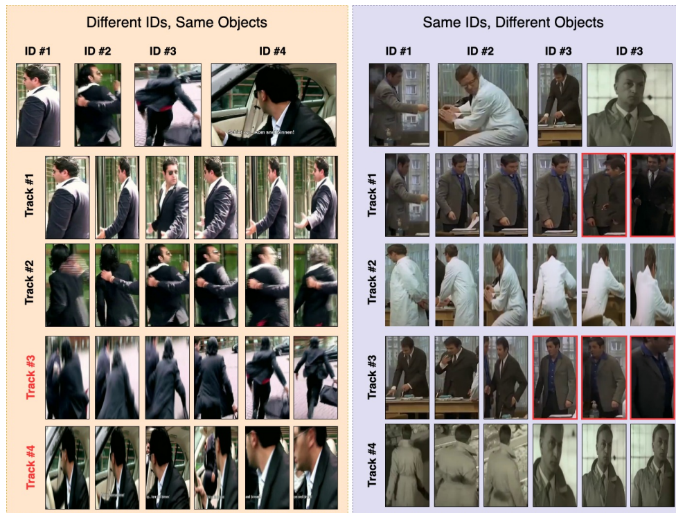
Figure 13: Tracking failures : Left : Different IDs, Same Objects - Tracks in red color are repetition of same earlier ID but assigned a new track. Tracks 1 and 4 are same IDs, and, tracks 2 and 3 are same IDs, but assigned different track IDs; Right : Same IDs, Different Objects - red boxes denotes switching of ID happened. Same id is assigned even if the object/actor is different.
