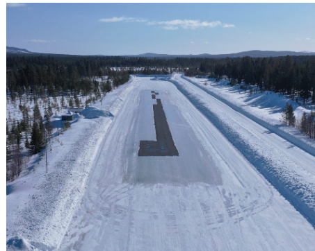
Figure 7: Mu-split test scenario. Image courtesy of Colmis AB.
