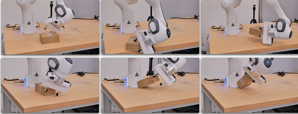
Figure 1: Long-horizon manipulation incorporates distinct non-prehensile skills: push-and-grasp (upper) and pivot grasp (blow). These skills are learned across diverse environmental settings with our proposed framework while employing the same reward function without any task-specific reward for non-prehensile manipulation. The videos are available at: https://youtu.be/4E74kLgeVas .
