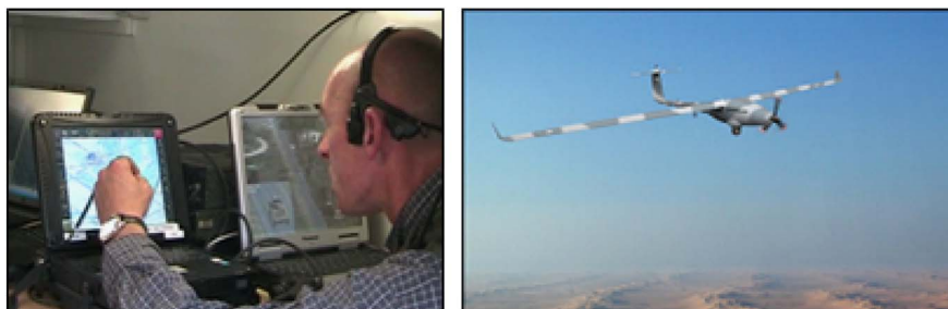
Figure 1 The patroller unmanned aerial vehicles (UAV) can detect targets at long range. With such UAV, the operator requests observation at preparation time or during mission execution
