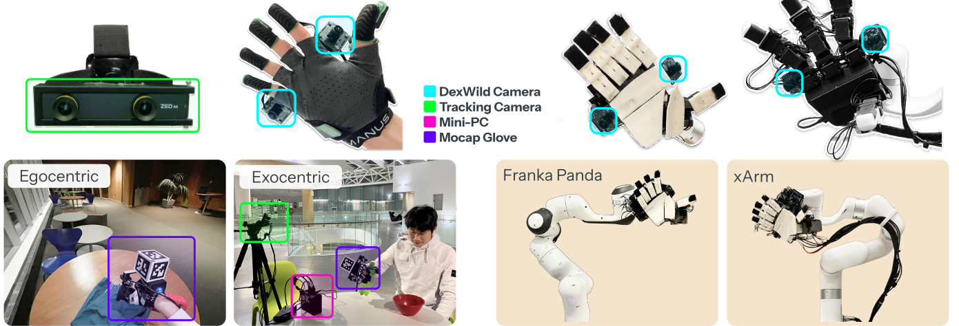
Fig. 2: Left: DexWild efficiently capture high-fidelity data using an individual’s own hands across various environments. Right: Robot hands are equipped with cameras aligned with the human cameras. We test DexWild on two distinct robot hands and robot arms.
