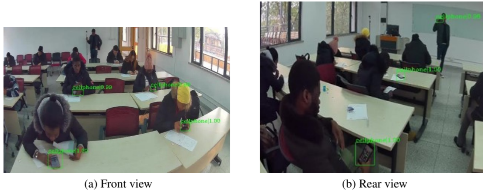
Figure 2: A front (a) and top-rear (b) view of a classified phone by the fine-tuned model
