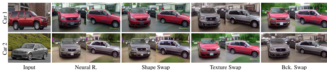
Figure 11: Real Image Manipulation: Given input images (1st col), we predict 3D properties and use our StyleGAN-R to render them back (2nd col). We swap out shape, texture & background in cols 3-5.
