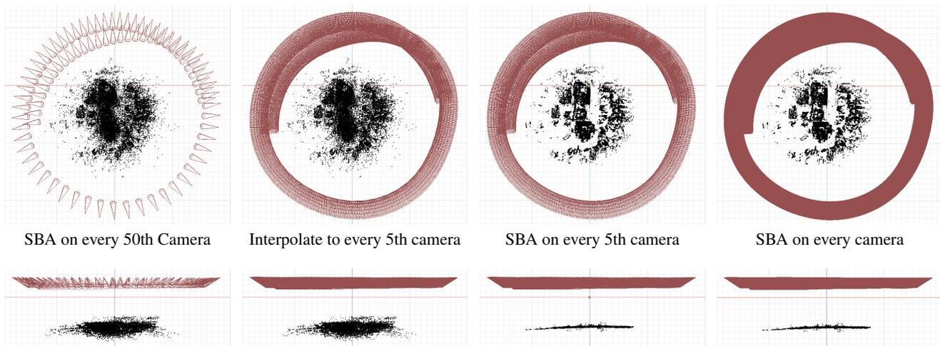
Figure 10. Hierarchical Sparse Bundle Adjustment on MAMI-I (sequences 152\*). Feature tracks are selected that span at least 50 frames. From left to right: 1. SBA run on every 50th frame (91 cameras total); 2. interpolate to provide every 5th frame, (991 cameras total); 3. SBA on interpolated cameras produces almost no change in cameras; 4. Interpolated all missing cameras and final SBA, almost no change.
