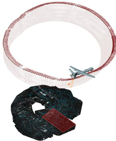
Figure 1. Aerial SfM: A UAV flies over a site and we wish to precisely estimate the camera pose at each image or video frame, a sparse 3D point cloud of observed landmarks, and optionally an orthorectified mosaic of the imagery.
