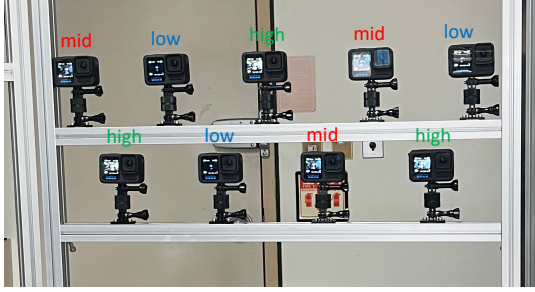
Figure 4. A camera rig for multi-exposure multi-view dataset. We use nine GoPro Hero 13 Black cameras arranged at two height levels with fixed spatial intervals. Each camera is synchronized to capture multi-view video simultaneously under three distinct exposure settings.
