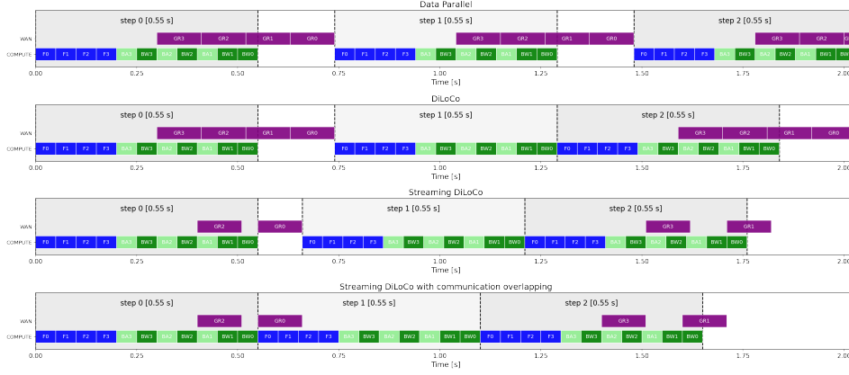
Figure 2: Simulation of a schedule interleaving forward passes (in blue), backward passes w.r.t. activations and parameters (resp. in light green and dark green), and (outer) gradient reduction (in purple).
