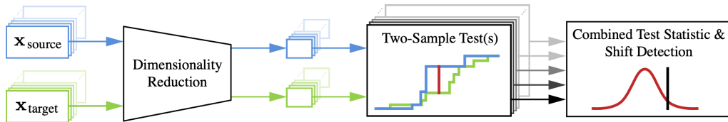
Figure 3: The procedure of detecting a dataset shift using dimensionality reduction and then a two-sample statistical test. The dimensionality reduction is applied to both the detection-training (source) and test (target) data, prior to being analyzed using statistical hypothesis testing. This figure is taken from (Rabanser et al., 2019).
