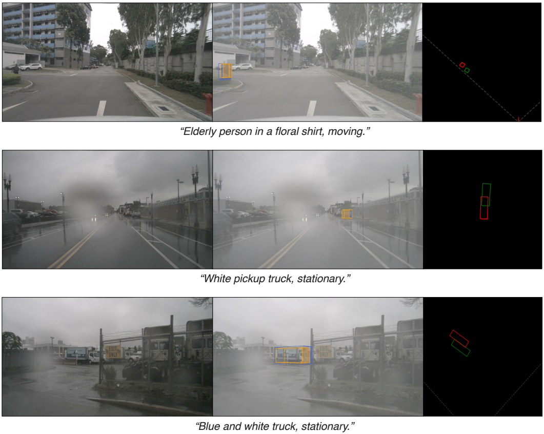
Figure 18: Failure cases of DriveLM-Grounding images. The error mainly attributes to incorrect depth. Each row has the original image (left), projected 3D box prediction and ground truth (middle), and BEV image (right). Blue box is the ground truth and Orange box is the prediction. In BEV images, Green box is the ground truth and red box is the prediction.
