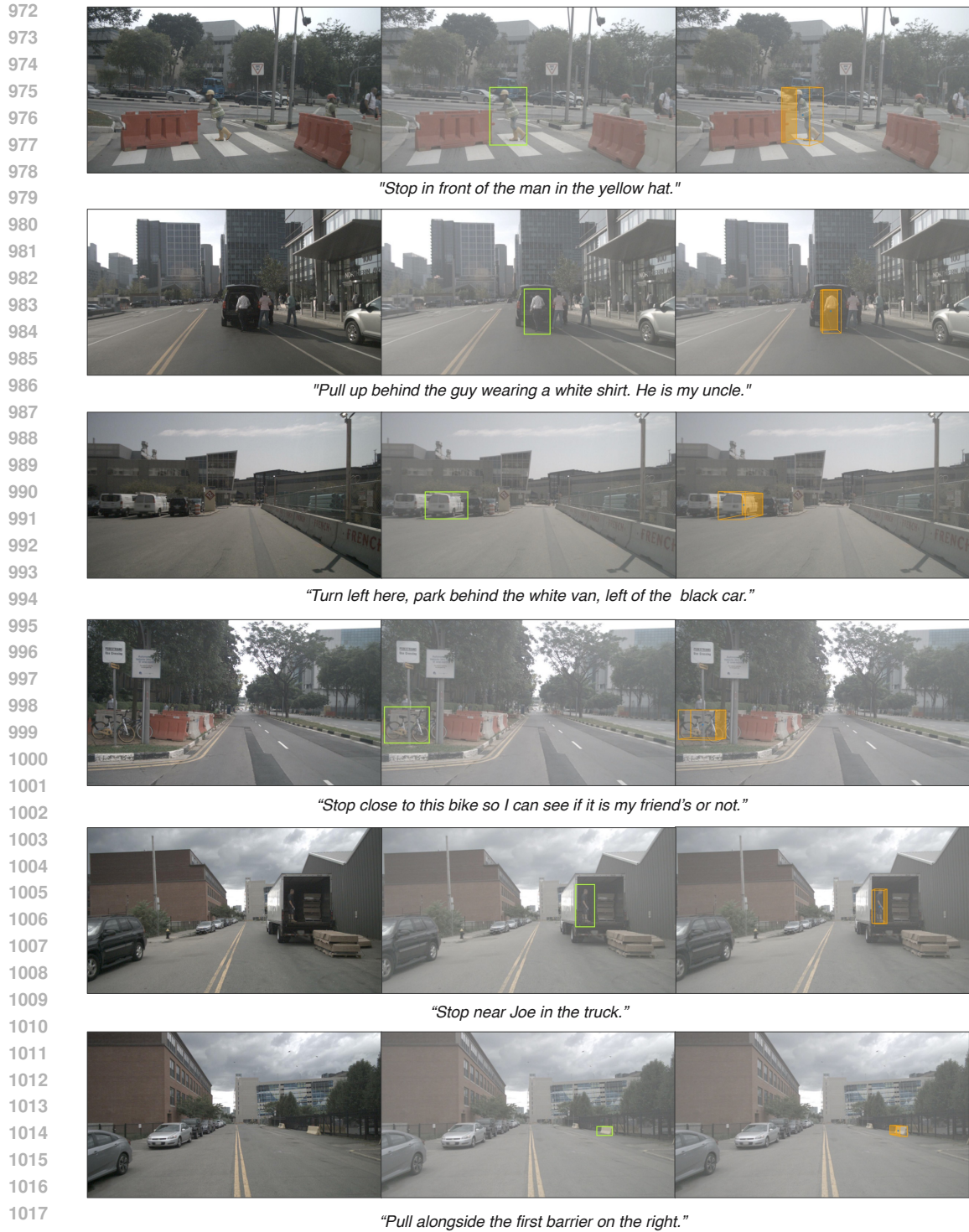
1019 Figure 9: CUBE-LLM visual chain-of-thought prompting inference. The first column is an input 1020 image, the second column is the 2D bounding box prediction, and the third column is the final 3D 1021 bounding box prediction prompted with the 2D prediction and text. 1022 1023 1024 1025
