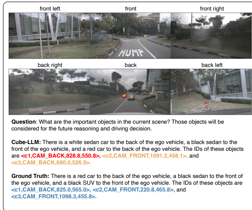
Figure 7: CUBE-LLM prediction on DriveLM-QA . Orange marks are predicted 2D points by CUBE-LLM . Blue marks are the reference marks and the corresponding bounding box in the ground truth answers. Red circle is the predicted object that does not agree with the ground truth.
