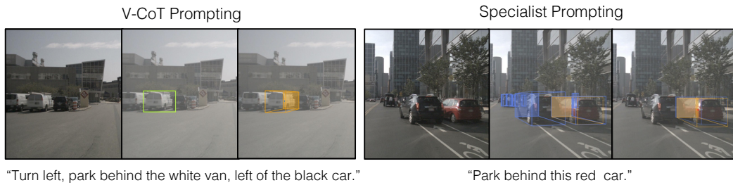
Figure 6: CUBE-LLM inference with prompting . Left : Visual Chain-of-Thought Prompting to reason in 3D step-by-step. Right : Incorporating specialist models to further improve localization of CUBE-LLM . Blue 3D boxes are the predictions of CenterPoint on corresponding LiDAR points.
