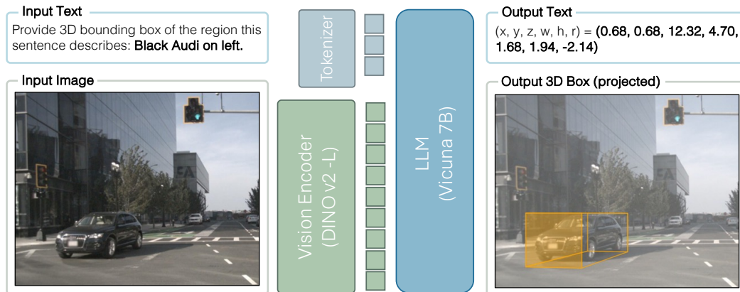
Figure 1: The overview of CUBE-LLM for 3D-grounding. The task requires a model to take an image, understand the input text prompt (e.g., “Black Audi on left.”) and ground it in 3D space.
