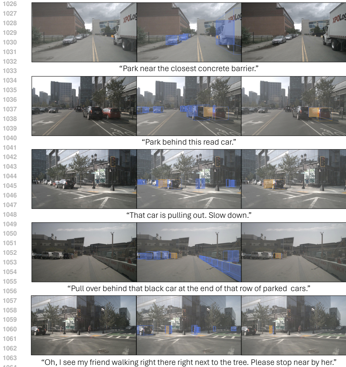
1066 Figure 10: CUBE-LLM visual prompting inference with specialist predictions. First column is an 1067 input image, the second column is the specialist predictions (blue) and the ground truth (orange), 1068 and the third column is the final 3D bounding box prediction of CUBE-LLM.
