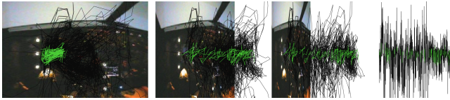
Figure 9: This figure shows the animated transition between the X/Y gaze view to the temporal view. This helps to detect how the selected eye movement occurred over time.
