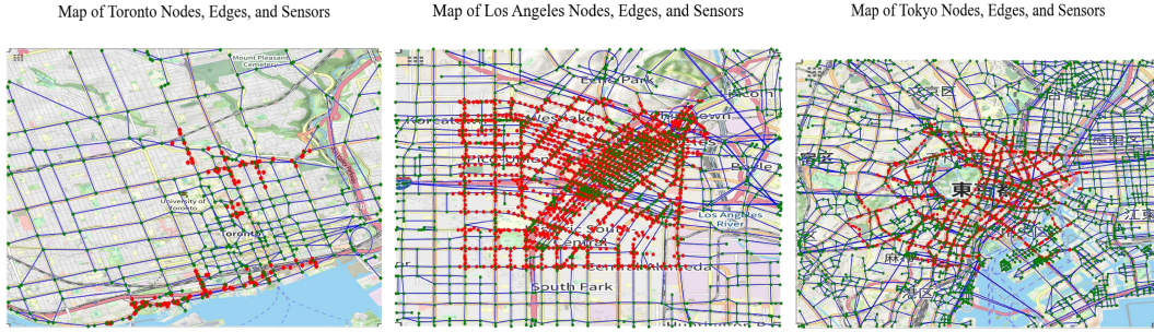
Figure 6: Map of Toronto, Los Angeles and Tokyo. The green points on the graph represent road nodes in OSM+, the blue lines represent road segments in OSM+, and the red points represent loop sensors. It can be seen that the road network information of OSM+ is very consistent with the actual ground truth. The loop sensors cover almost all the nodes in the central area of the city, which can better reflect the traffic flow information of the city.
