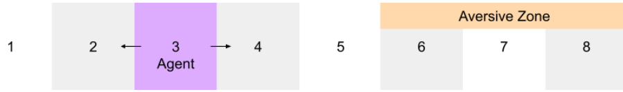
Figure 1: Diagram of the Conditional Avoidance environment. The agent, a neural organoid, is embodied in a 1D world. Its decision to move left or right is decoded from neural activity. Entering the aversive zone triggers unpredictable punishment, driving the agent to learn a world model where that region is associated with negative outcomes.
