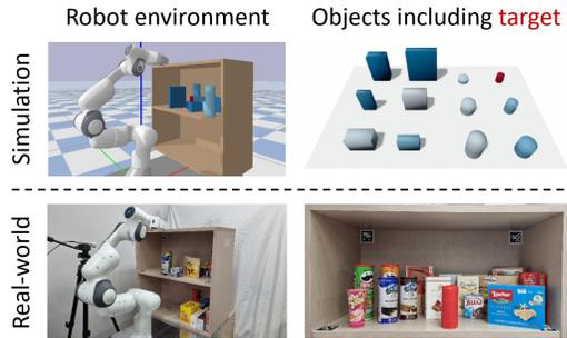
Figure 4: The left column shows the simulation and real environments, and in the right column, objects used in each environment are visualized. In particular, the target object is marked in red in the simulation; the red-taped can is the target object in the real experiment.
