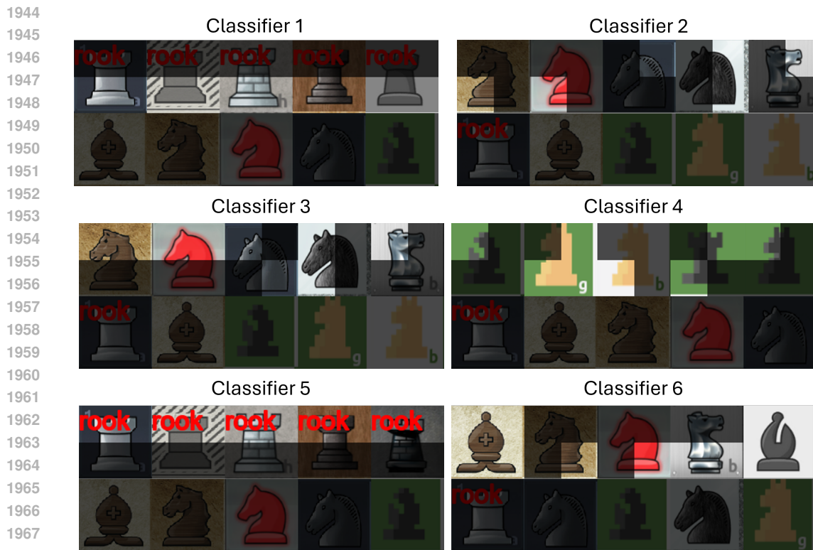
Figure 22: Example image segmentations based on the concept detectors learned for the model correction experiment. Top rows illustrate pictures with the concept and bottom rows illustrate pictures without. Classifier 5 clearly detects the watermark.
